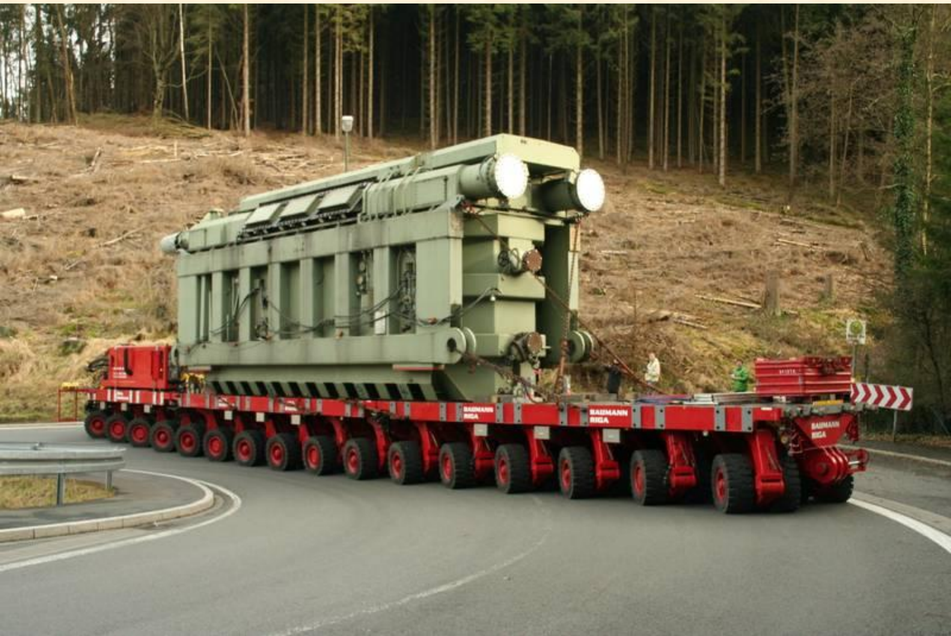
Round the bend slowly, note the front & rear section wheels steer in opposite way.
