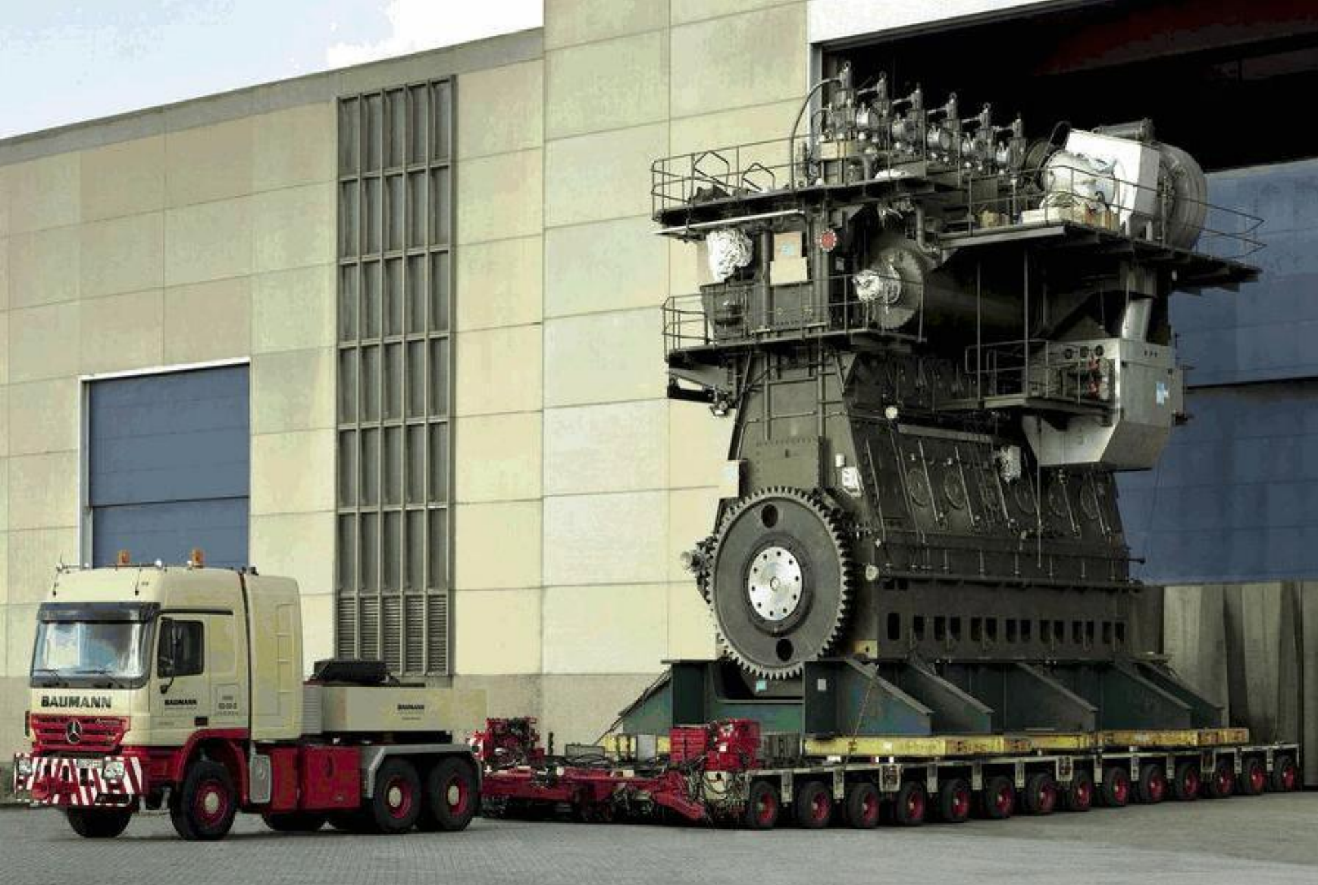
Marine diesel ( about 75 MW or 100,000 hp ) for container ship or oil tanker
